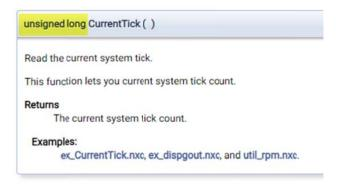
In other words, calling <code>CurrentTick()</code> returns a 32-bit number. That number does not represent the time that's elapsed. Rather, it's the crystal's current tick value. One has to call <code>CurrentTick()</code> once more, and compute the difference between the second and first call. This difference reflects the number of milliseconds that has elapsed between the two calls. A 32-bit timer can measure quite a long time:
