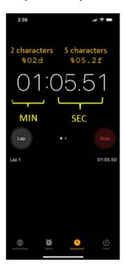
On the left is an annotated screenshot of an iPhone's stopwatch app. The format is MM:SS.XX where MM is a 2-digit number for minutes. This means it will increment from 0 to 59 minutes. SS.XX is real number that represents the number of seconds. SS will increment from 0 to 59 seconds. XX denotes 10<sup>th</sup> of a second and increments from 00 to 99.
