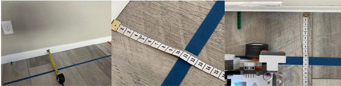
Blue tape is 10 cm from wall baseboard. Ultrasonic sensor shows portside sensor at 10 cm
