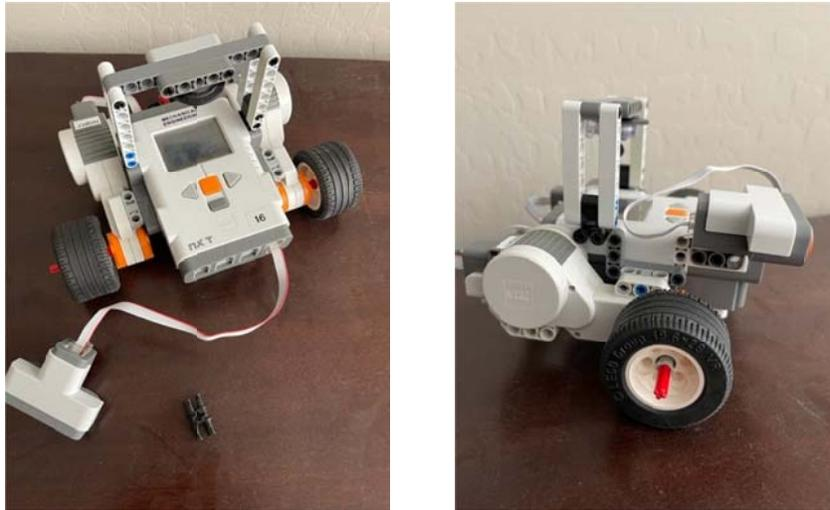
Figure: Technic Part 32138 Double Pin with Axle (left) attaches ultrasonic sensor to Domabot (right)
