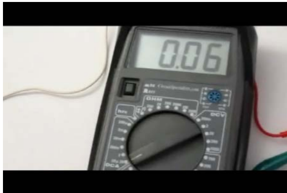
Figure C: Ammeter close up reveals 6 milliamp running current at no load and lithium NXT battery at 100% motor speed
