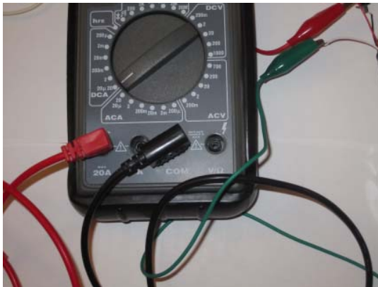
Figure 2A: This multimeter is set for a 20 Amp ammeter (see dial and red lead). The black lead is connected to COM
