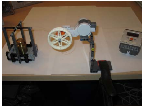
Figure B: The winch (motor and wheel) are clamped to overhang from a desk. The mass can then suspend from the desk.
