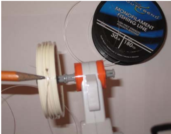
Figure 4I: Drill hole in wheel and mount on motor axle
