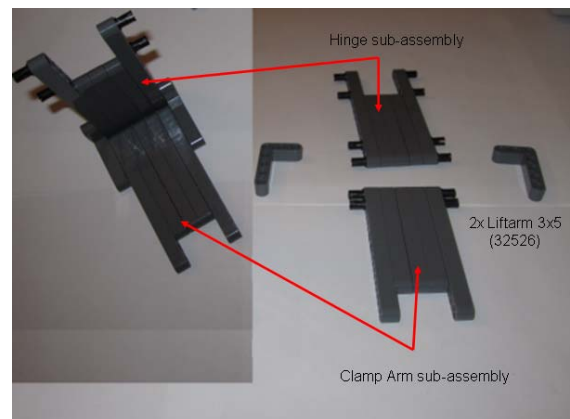
Figure 2C: Right shows constructed clamp arm (from Step 1) and hinge (from Step 2). Left shows how the two are connected with liftarms
