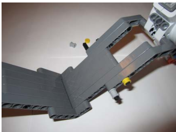
Figure 4G: Thread and bush the axles
