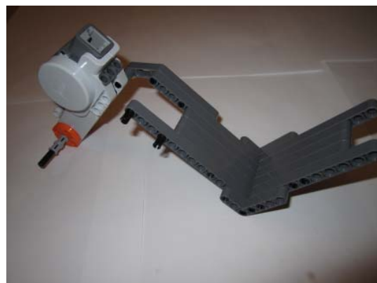
Figure 4B: Mount motor arm and thread motor axle
