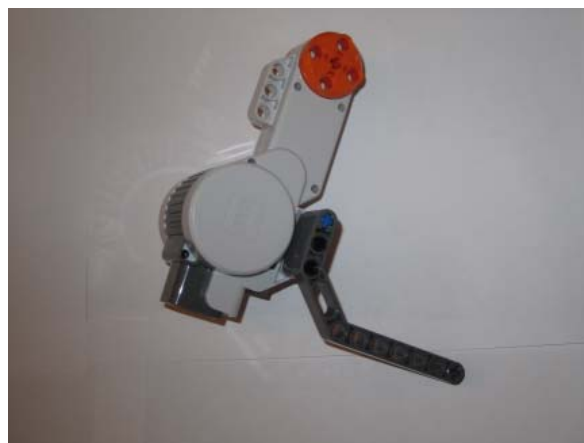
Figure 3C: Attach Beam 3 to motor and then liftarm
