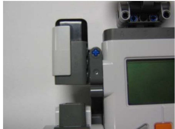
Figure 6D: Attach gyro to the left side of NXT Brick
