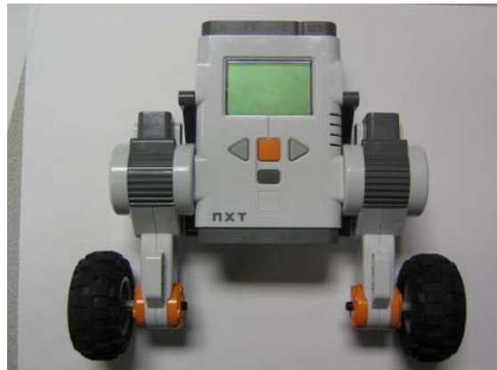
Figure 3E: Attach Wheel/Axle to Motors
