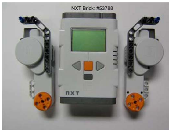
Figure 2D: Attach Motors to NXT Brick
