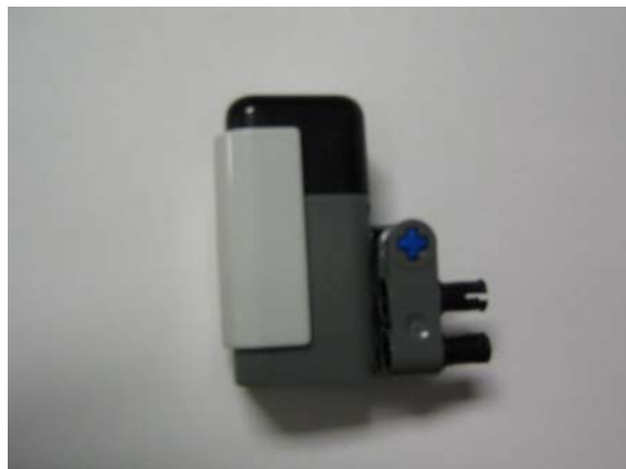
Figure 6C: Attach connector to gyro
