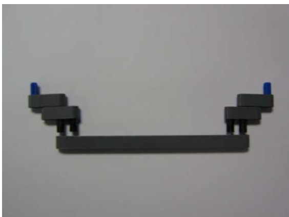
Figure 5C: Attach arm from 5A to 5B
