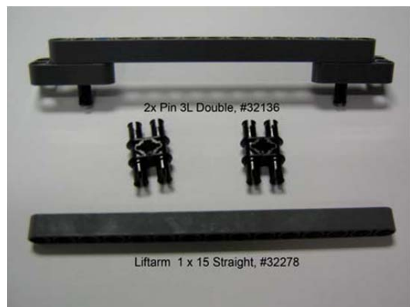
Figure 4F: Add another liftarm and connect with pins
