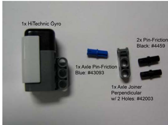
Figure 6A: Gyro mount components
