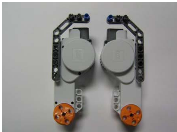
Figure 2C: Attach Arms to Motors
