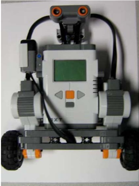
Figure 7B: Wire Gyro to Sensor Port 1 (ignore ultrasonic sensor)
