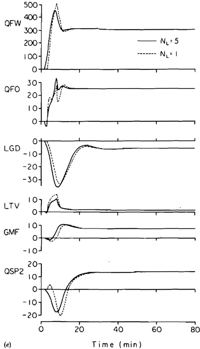
Figure 3. Closed-loop responses: (a) main steam pressure TP, (b) generator output MW, (c) controlled variables MST, TPL, RHT and NOX, (d) measurable outputs TISH, TF, TECO and O<sub>2</sub>, (e) control variables QFW, QFO, LGD, LTV, GMF and QSP2.
