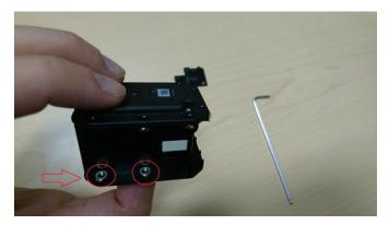
• Then tie up the "fixture plate" with the 3M bolts
