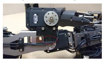
• Tie up the wheel to the MX-28T by using (2M bolts)
