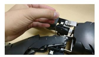
• Fix the "fixture plate" onto the MX-28T Dynamixel
