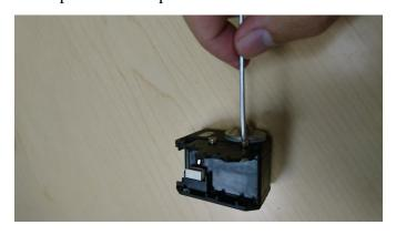
• Remove the little hatch that holds the cable
