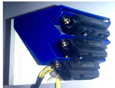
Fig. 3. Infrared range sensor system.
