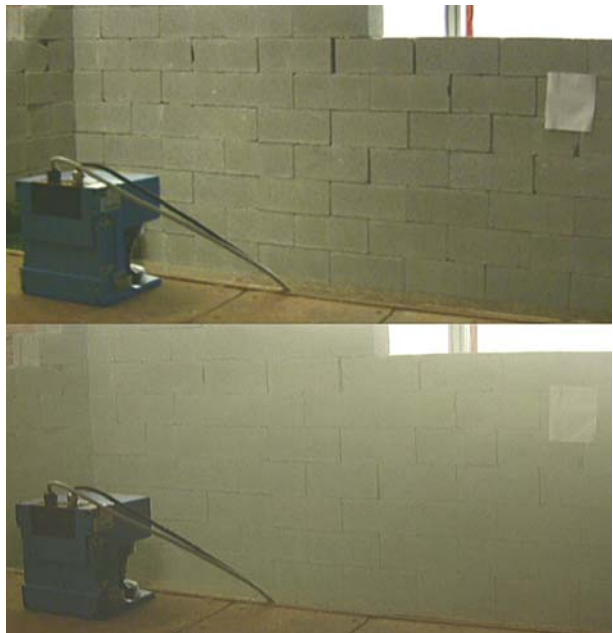
Fig. 5 To characterize the SICK LMS200, the sensor was placed inside the testing environment and pointed toward a white sheet of paper placed 3m away. 500 data points were recorded without smoke ( top ) and in smoke with a visibility of approx. 15m ( bottom )
