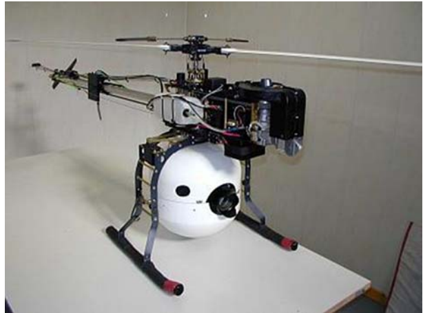
Fig. 7 The SR100 robotic helicopter from Rotomotion, Inc. The SR100 is sold as a fully robotic package capable of automated take off, landing, and GPS waypoint following
