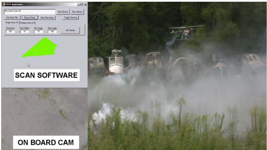
Fig. 8 The LMS200 was attached to the bottom of the SR100 helicopter and flown over smoke. Results showed that the LMS200 reflected off of the smoke, but was still able to locate flat terrain to land
