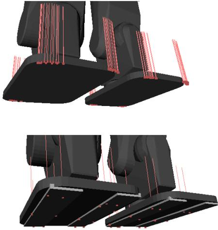
Fig. 4. Comparison of contacts detected with trimesh-primitive (upper) collision vs. primitive-primitive (lower) collision. Fewer discrete contacts reduce computational burden during convex hull generation.
