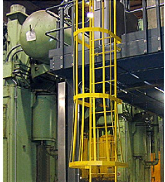
Fig. 1. An example of a ladder with safety cage for equipment access.
