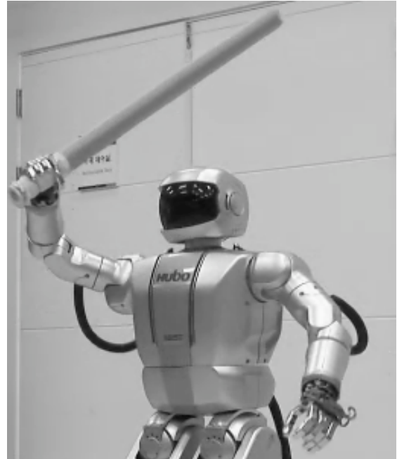
Figure 1: Hubo is currently limited to shape adaptive grasp
