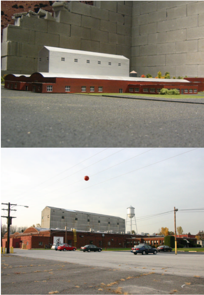
Fig. 3 The V&V environment compared to the 1/87th scale T&E environment. The T&E facility was created to closely approximate the helicopter development range in order to draw a continuous path between laboratory testing and real-world flights.
