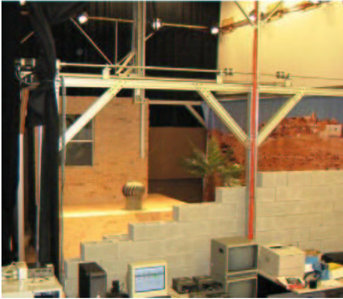
Fig. 4 Systems integrated sensor test rig (SISTR). SISTR provides a stage for testing and evaluating sensor and control algorithms in a scaled environment. The 6 DOF gantry that comprises SISTR can be programmed through model adaptive control to mimic the flight of UAVs.
