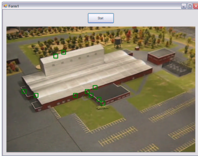
Fig. 6 Kanade Lucas feature detection implemented on video of the scaled T&E environment. The algorithm successfully detected features such as the corner of buildings and windows. These features are consistent between the model and the real world, allowing for a more strict comparison of the scaled and full sized environments.
