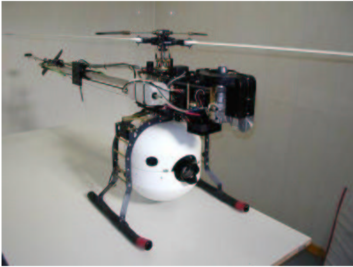
Fig. 5 The SR100 helicopter from Rotomotion, Inc. The SR100 is sold as a fully robotic package capable of automated take off, landing, and GPS waypoint following.
