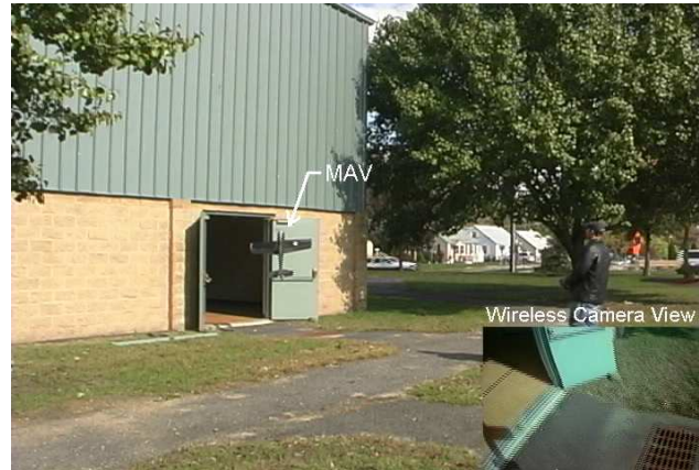
Figure 1: A fixed-wing MAV transitions to hovering mode to gently maneuver itself through a small opening of an urban structure. Inset : once inside, the on-board wireless camera is used to capture and transmit surveillance images.
