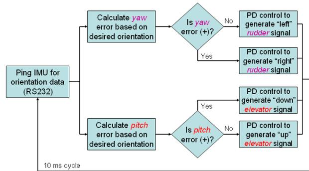
Figure 8: Flow chart describing the autonomous hovering code.
