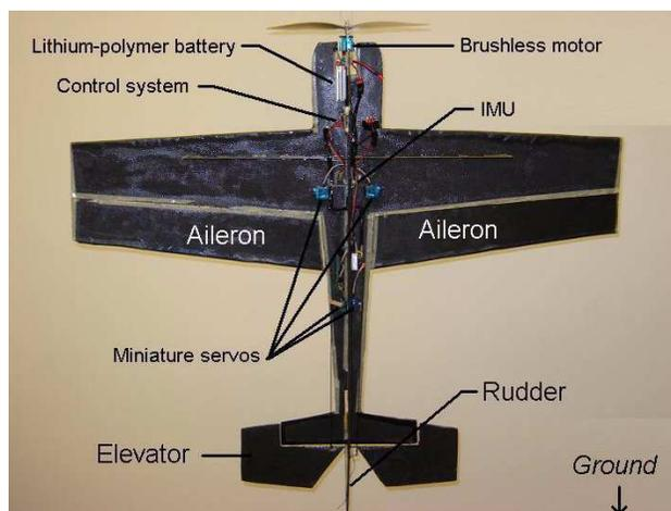
Figure 2: The fixed-wing prototype in its hovering orientation.
