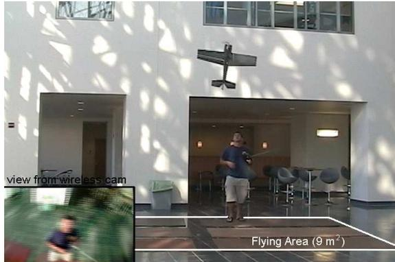
Figure 9: MAV performing a *hands-off* autonomous hover in and urban structure. *Inset*: a shot from the MAV’s bellycam is shown.
