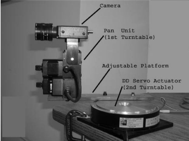
Figure 1: Experimental Platform: The camera has rotational redundancy and can be positioned either by the pan-tilt unit, turntable or both
