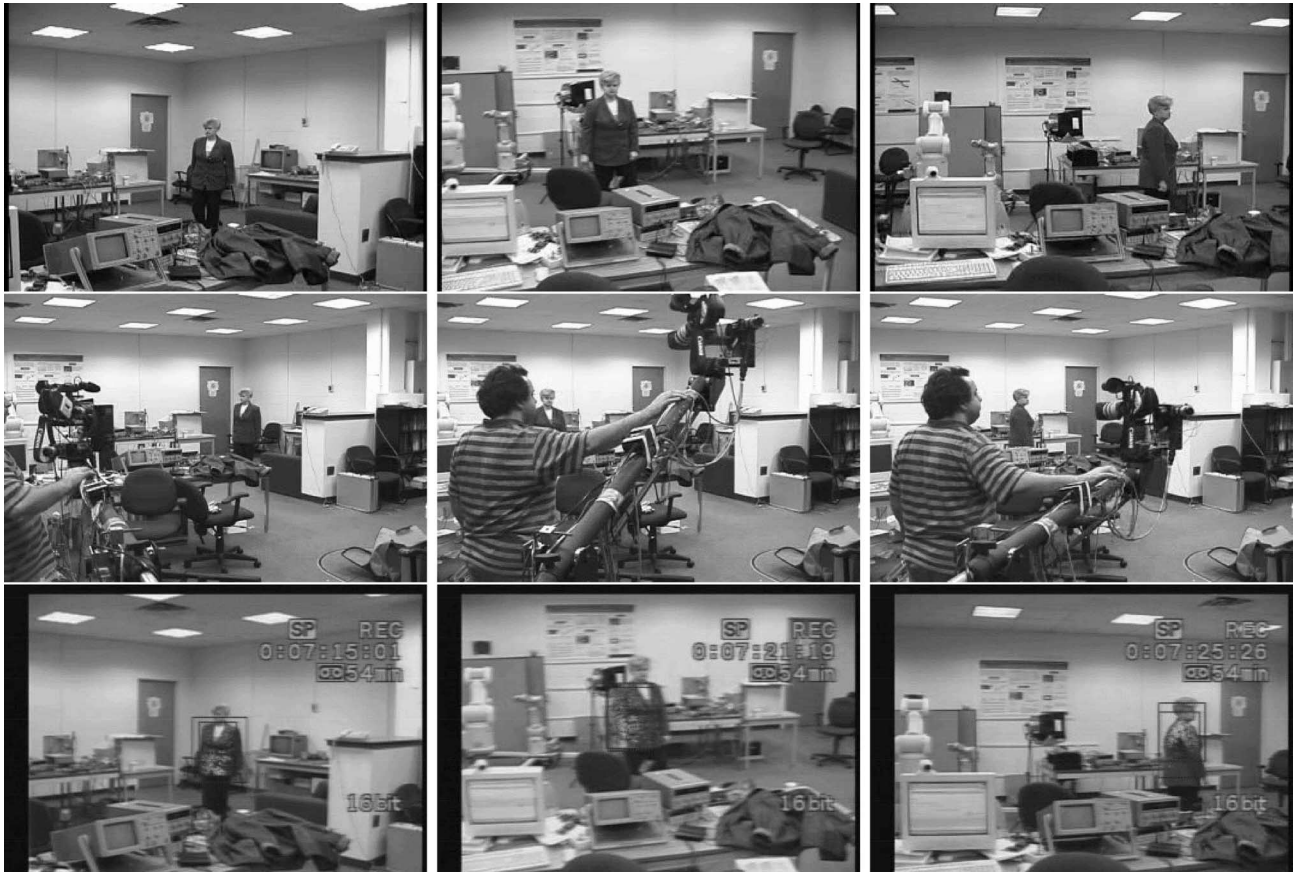
Fig. 8. Three sequential images from videotaping the feedforward controller experiment. Camera field-of-view shows target is tracked top row . Boom manually controlled middle row . Working program bottom row .
