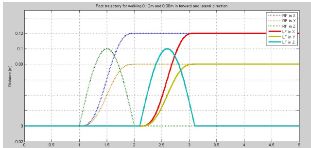
Fig. 13. Right and left foot trajectories for moving to (0.154m, 0.08m) in X and Y direction, respectively
