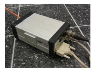
How to connect with Ethernet Open RiSCAN, Under Tools select "Scanner Search...", and search for the scanner in the appropriate range of IP addresses.
