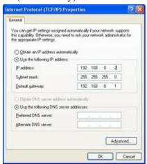
Open a DOS window and ping the new address of the communications box to verify connection. Make sure that RiSCAN is setup properly as in Keith Sevcik's tutorial
