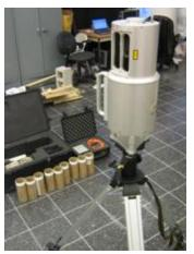
Connect the serial and the parallel cables between the scanner and the communication box, and attach both devices power cords to a 12 volt power source. Connect the cross over ethernet cable between the communication box and the laptop computer.
