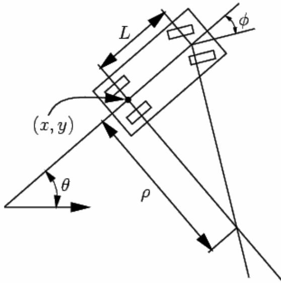
$$\begin{aligned}\dot{x} &= V \cos \theta \\ \dot{y} &= V \sin \theta \\ \dot{\theta} &= \frac{V \tan \phi}{L}\end{aligned}$$
