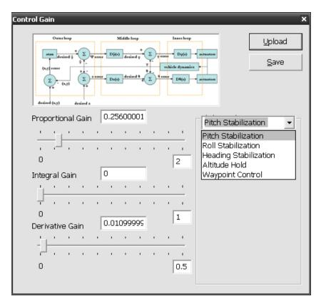
All the gain values are adjustable but the combo box on the right are pre-set gain values for different control problems. Click the "Upload" button to upload the new gain values to the MNAV. Also you can save your modified gain values to the <code>gainsetting.txt</code> files but using the "Save" button.
