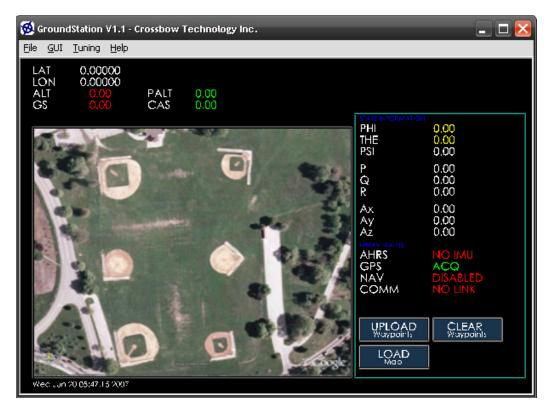
Enclosed with version 1.0+, the Groundstation comes with a Open Glass Cockpit found under the "GUI" menu. The system must be configured before using it (see above). The cockpit looks like the following:
