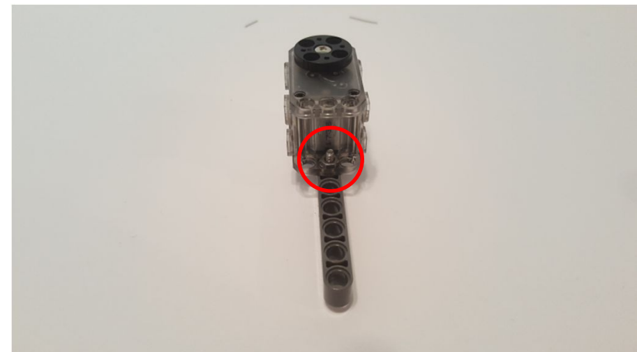
Alternative view of Step 1C. Red circle shows fastened M2.5 nut
