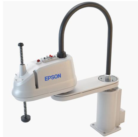
**Figure A:** Reference frames using Denavit-Hartenberg convention (left). Many manufacturing robot companies like Epson (right) offer SCARA products. Video of operation:
