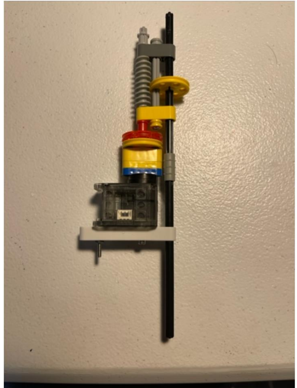
Connect Motor Drive mount onto Thin Beam 3 (blue). Use Axle Connector to join lower and upper Axle 12 parts
