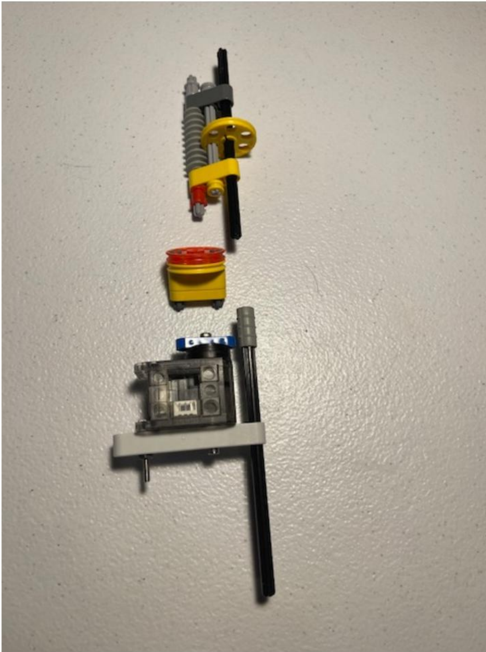
Screw Thin Beam 3 (blue) onto XL-320. Screw XL-320 to mount onto Beam 5. Thread Axle 12 through Beam 7
